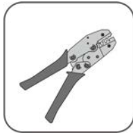
Tube terminal crimping tool (0.5 mm 2 –1.0 mm 2 )
