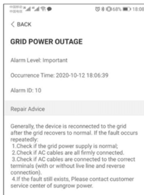
figure 7-9 Detailed Fault Alarm Information
