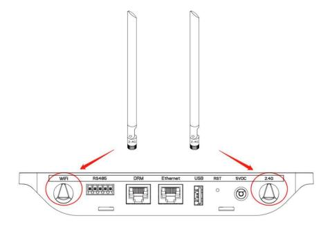
**Note:** If the SLS installation location is inside the metal box or under the metal / concrete roof, extended 2.4G cable or 2.4G sucker antenna will be suggested, which can be purchased from Solenso or local electrical store (Please contact Solenso's Tech. support team for the detail type of the cable or antenna at info@solenso-global.com/ info.eu@solenso-global.com).
