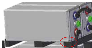
Wrong, the weak point is on the cabinet ledge, see the highlighted area marking
